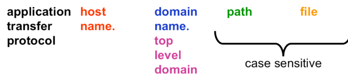
Figure X: Anatomy of a Web Address. The URL displayed says “use the web (http) to find a host server named “www” in the “nytimes.com” network, look in the “tech” directory, and access the “indx.html” file.
